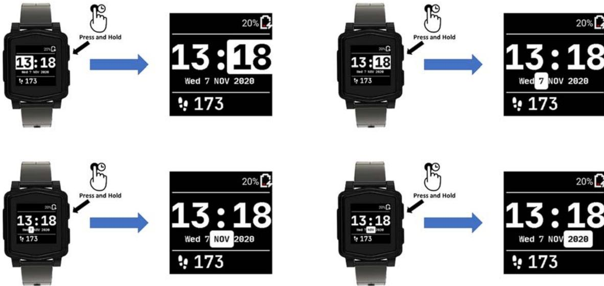
Figure 7 Press and hold Button 1 to rotated between the fields to edit.
